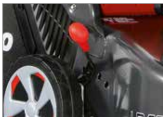
Practical, lever-operated cutting height adjustment system.
