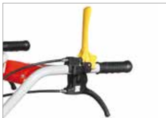
Handlebar-mounted gear lever.
